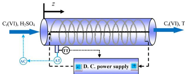
Fig. 1. Cr(VI) removal system and its control implementation.
