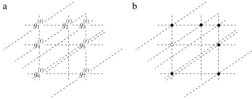
**Fig. 1.** A two-dimensional example for three projection directions (signal-recording lines indicated by dashed lines). (a) The grid  $G^{(t)}$ , and (b) a possible solution  $\vec{x}^{(t)}$  representing a set of particles that are consistent with the projections (black and white dots corresponding to  $\xi_i^{(t)} = 1$  and  $\xi_4^{(t)} = 0$ , respectively).
