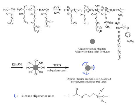
Scheme 1. Synthetic scheme of organic fluorine and nano-SiO<sub>2</sub> modified polyacrylate emulsifier-free latex.
