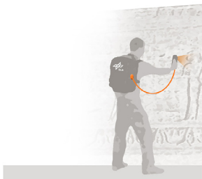
Fig. 1. The portable DLR 3D-Modeler used for cultural heritage preservation.
