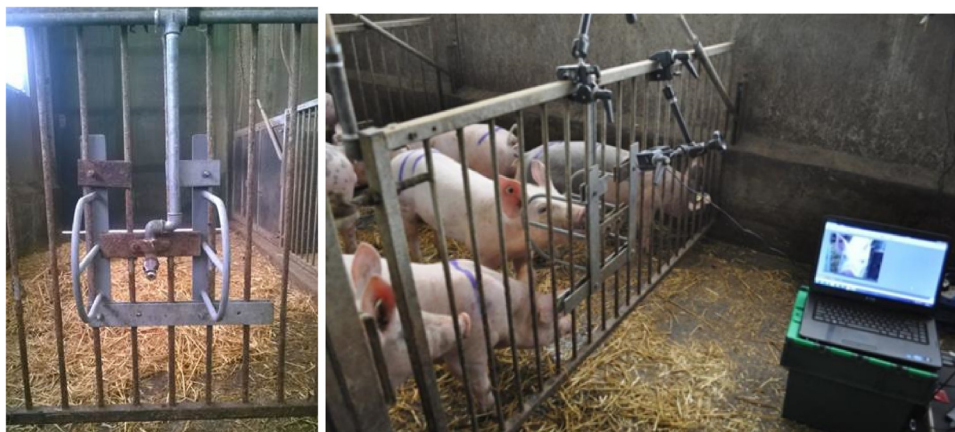
Fig. 2. Photographs showing the modified drinking nipple (left) and the arrangement of the webcam behind it (right).
