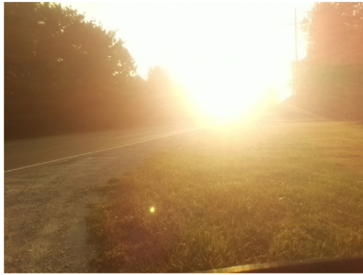
Fig. 1. Image of direct sunlight using automatic exposure correction. Road lines are difficult to see in direct sunlight and the image is slightly discolored.
