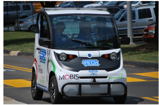
Fig. 3. Lawrence Technological University's Autonomous Campus Transport (ACTor) vehicle driving autonomously on parking lot roadways.
