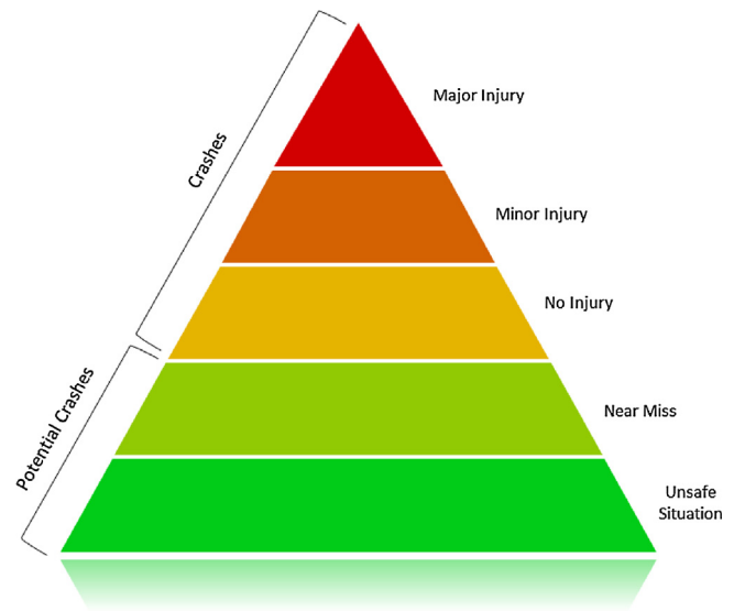
Fig. 1. The Heinrich Triangle describes crash events in terms of injury severity and near crash or potential crash events in terms of risk. Events at the base of the triangle happen more frequently.
