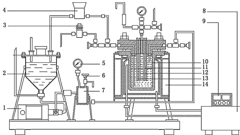
**Fig. 1.** Schematic diagram of the experimental setup for deep ocean corrosion study. (1) Booster pump, (2) artificial seawater pot, (3) discharge port, (4) inching valve, (5) pressure gauge, (6) valve, (7) buffer pot, (8) thermostatic bath, (9) temperature monitor, (10) thermocouple, (11) reference electrode, (12) counter electrode, (13) working electrode, and (14) pressure kettle.
