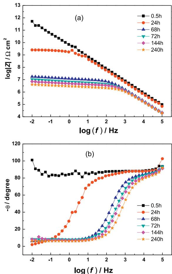
**Fig. 2.** EIS results for E44 coating at normal hydrostatic pressure (a) Nyquist plot; and (b) Bode plot.
