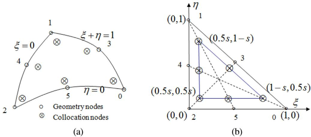
Fig. 2. 6-node discontinuous triangular element.
