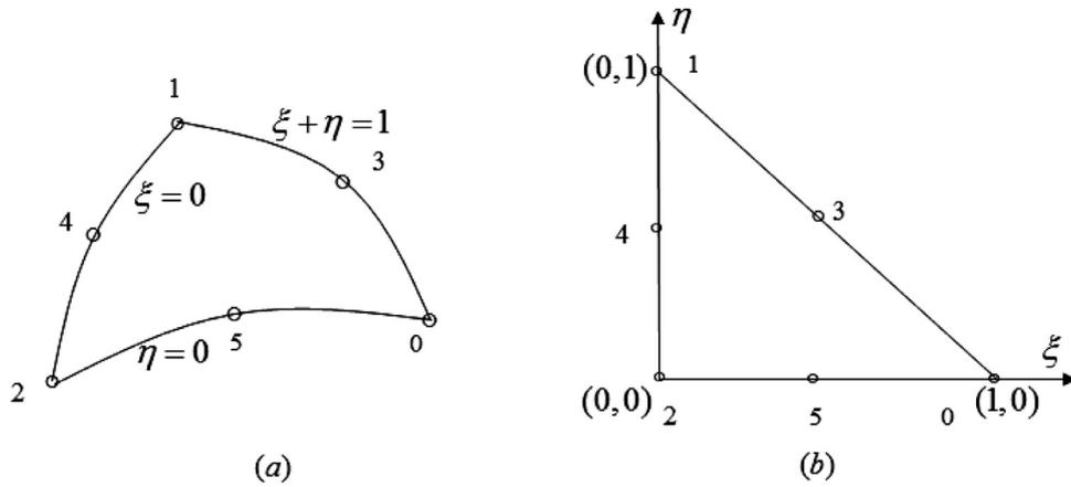
Fig. 1. 6-node continuous triangular element.
