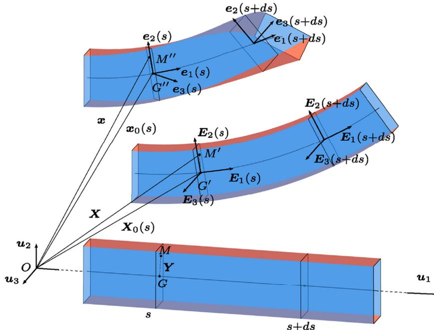
Fig. 1. Kinematics of the geometrically exact beam model.
