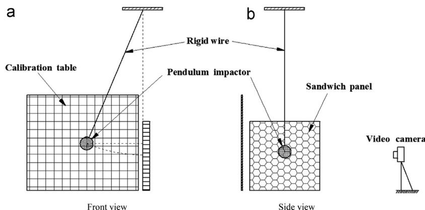
Fig. 2. Pendulum-impacting system.
