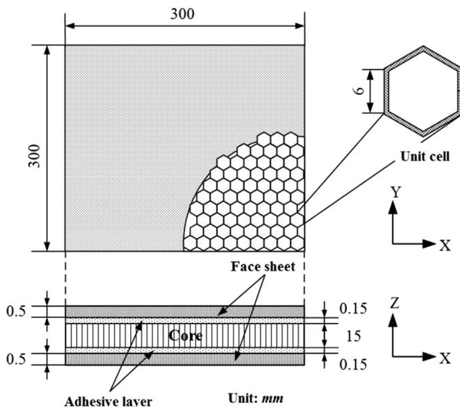
Fig. 1. The honeycomb sandwich panel.
