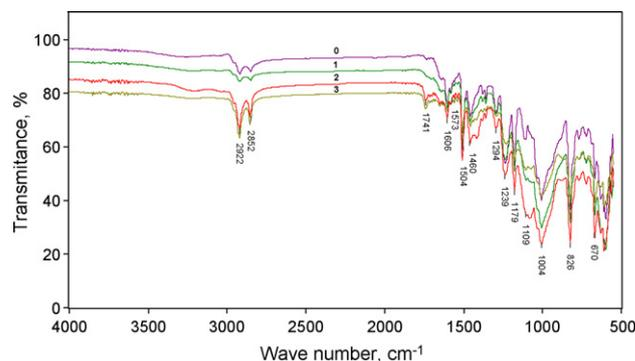
Fig. 2. FTIR spectra of epoxy coatings subjected to sulphuric acid aqueous solutions for 1080 h: 3%—curve 1, 10%—curve 2, and 20%—curve 3 (unaged coating—curve 0).
