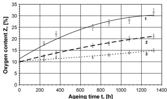
Fig. 1. Oxygen content in epoxy coating surface layers subjected to the action of sulphuric acid aqueous solutions: 3% (curve 3), 10% (curve 2), and 20% (curve 1).
