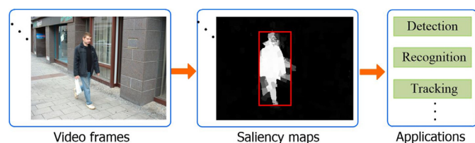
Fig. 1. Illustrating saliency's role of reducing the search space for further processing on the video surveillance systems.
