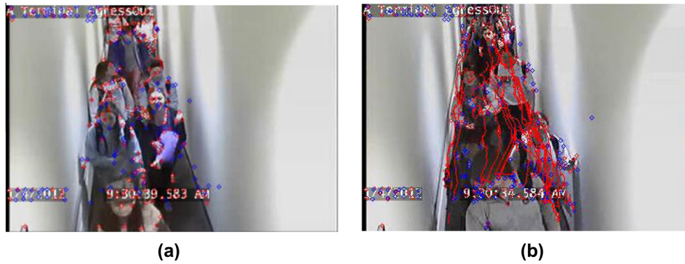
Fig. 1. Results of feature tracking. (a) Features detected in the image. (b) Point tracks extracted from a video sequence.
