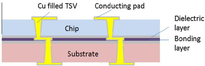
Fig. 1. Illustration of MEMS 3D integration and wafer-level packaging with a typical TSV technology.
