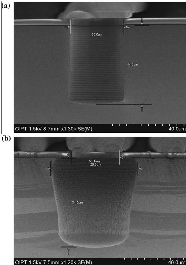
Fig. 2. Tapered via fabrication by two-step etching (a) after high-rate Bosch etch (18  $\mu\text{m}/\text{min}$ ); (b) subsequent  $\text{SF}_6/\text{O}_2$  isotropic etch, 80° profile at a 30  $\mu\text{m}$  via, but overhang at top.
