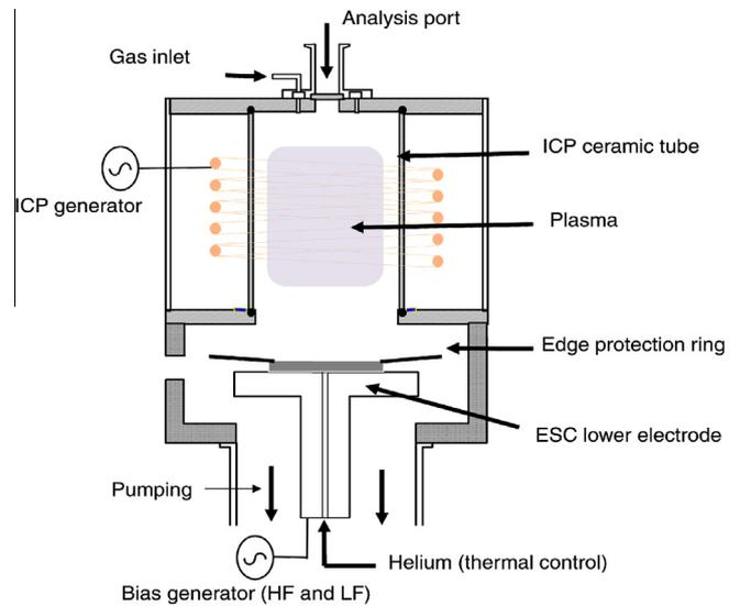
Fig. 3. Schematic of an ICP etch system.
