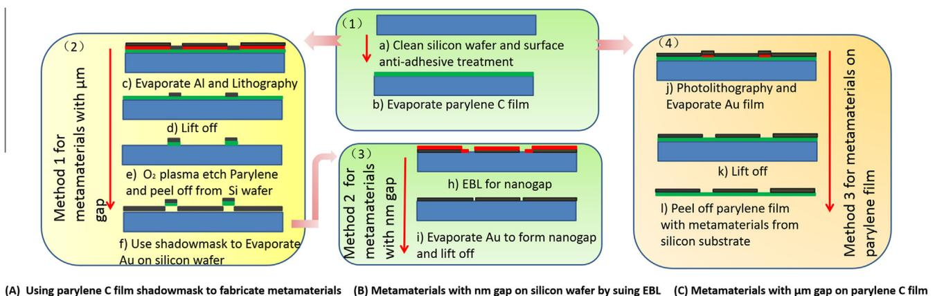
Fig. 1. The fabrication processes of the flexible, large-area metamaterials with micro/nanogap and high  $Q$  value.
