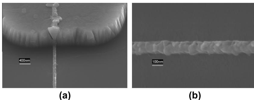
Fig. 2. SEM images of sample No. 3: (a) contact between the nano-size wire and the pad and (b) top view of the Al wire.
