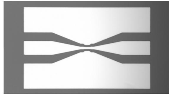
Fig. 3. Thru de-embedding test structure.
