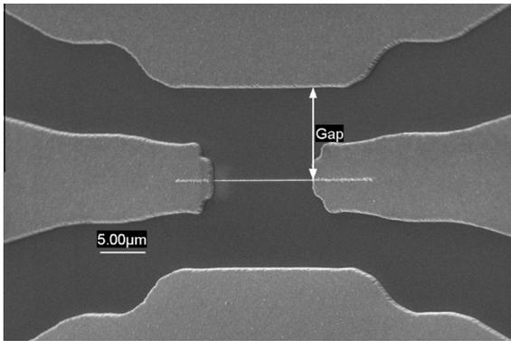
Fig. 1. SEM image of a nano-size Al wire embedded in a CPW structure.
