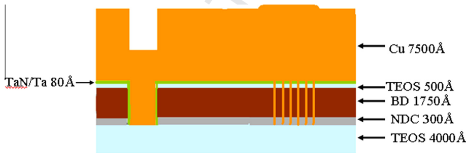
Fig. 2. The schematic of patterned copper wafer used in this experiment.
