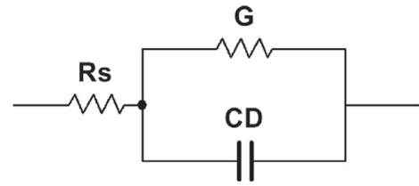
Fig. 1. RC small signal equivalent RTD model [30].
