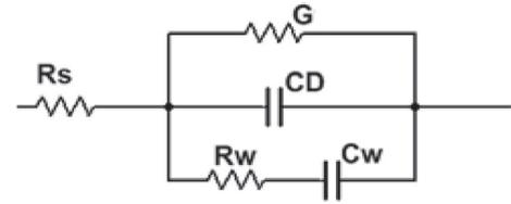
Fig. 2. Series/parallel double RC network [31].
