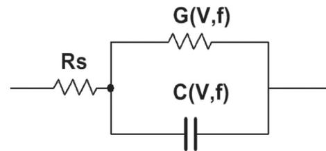
Fig. 3. The large signal and equivalent circuit model [32].
