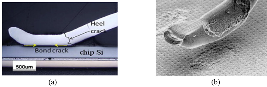
Fig. 1. (a) Locations of bond wire heel and bond crack [6]. (b). Wire bond lift-off failure which is the result of bond crack [7].
