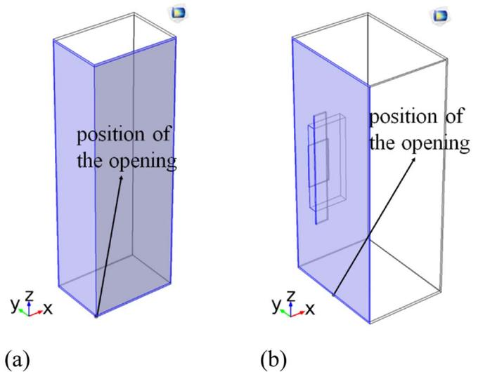
Fig. 1. Illustration of the investigated geometries; (a) empty enclosure, (b) enclosure with components inside (symmetry faces are shown in blue). (For interpretation of the references to color in this figure legend, the reader is referred to the web version of this article.)
