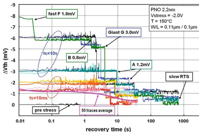
Fig. 1. Recovery traces recorded after repeated gate stress pulses with  $t_s = 10$  ms and 10 s pulse length. Four different defects (named A, B, F, G) with different capture- and emission-time constants and step heights are charged. Also shown is an average over 50 recovery traces after  $t_s = 10$  ms, showing the exponential distribution.
