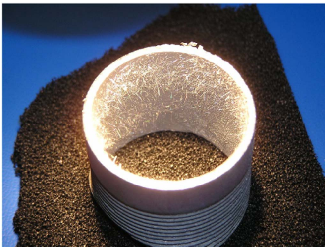
Fig. 2. Hot dip galvanized steel pipe with extensive zinc whisker formation [3]. Courtesy of NASA Electronic Parts & Packaging (NEPP) Program.
