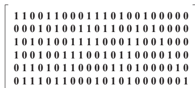
Fig. 1. Parity check matrix H for the (22, 16) SEC-DAEC code in [9].
