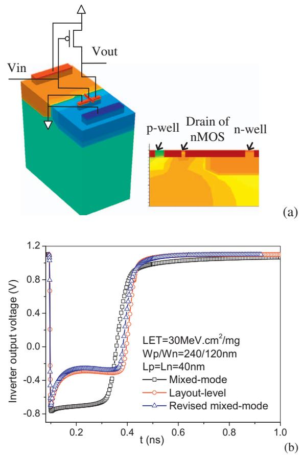
Fig. 3. Comparison of TCAD simulated SEE response of the  $W_p/L_p = 240/40$  nm and  $W_n/L_n = 120/40$  nm inverter produced by mixed-mode, revised mixed-mode and layout-level simulations.
