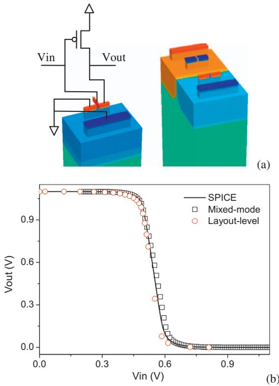
Fig. 1. TCAD structures for mixed-mode and layout-level simulations of a  $W_p/L_p = 240/40$  nm,  $W_n/L_n = 120/40$  nm inverter (a); TCAD and SPICE simulated transfer characteristics (b).
