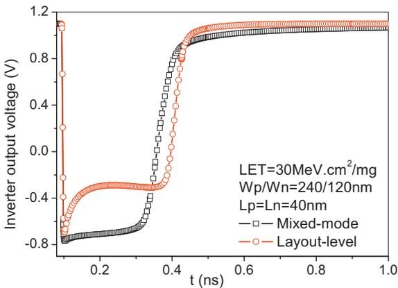
Fig. 2. Comparison of TCAD simulated SEE response of the  $W_p/L_p = 240/40$  nm and  $W_n/L_n = 120/40$  nm inverter produced by mixed-mode and layout-level simulations.
