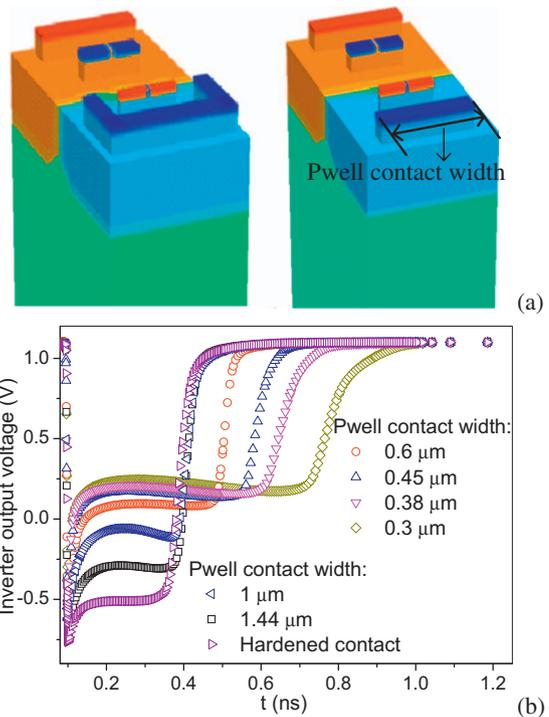
Fig. 4. 3-D TCAD structures of inverter with hardened p-well contact and strip contact of various contact widths (a); TCAD simulated output voltage pulses for  $LET = 30 \text{ MeV} \cdot \text{cm}^2/\text{mg}$  strike at the nMOS drain region (b).
