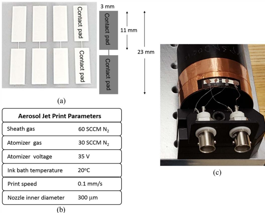
Fig. 1. (a) Four completed samples on a single substrate and the dimension of each sample. (b) Aerosol-jet parameters for printing the trace. (c) Setup for investigating the effect of tensile stress bending.
