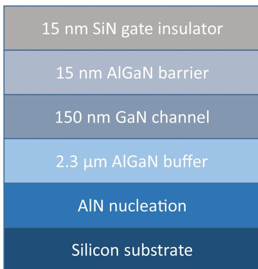
Fig. 1. Schematic structure of the described devices (see details in [10]).
