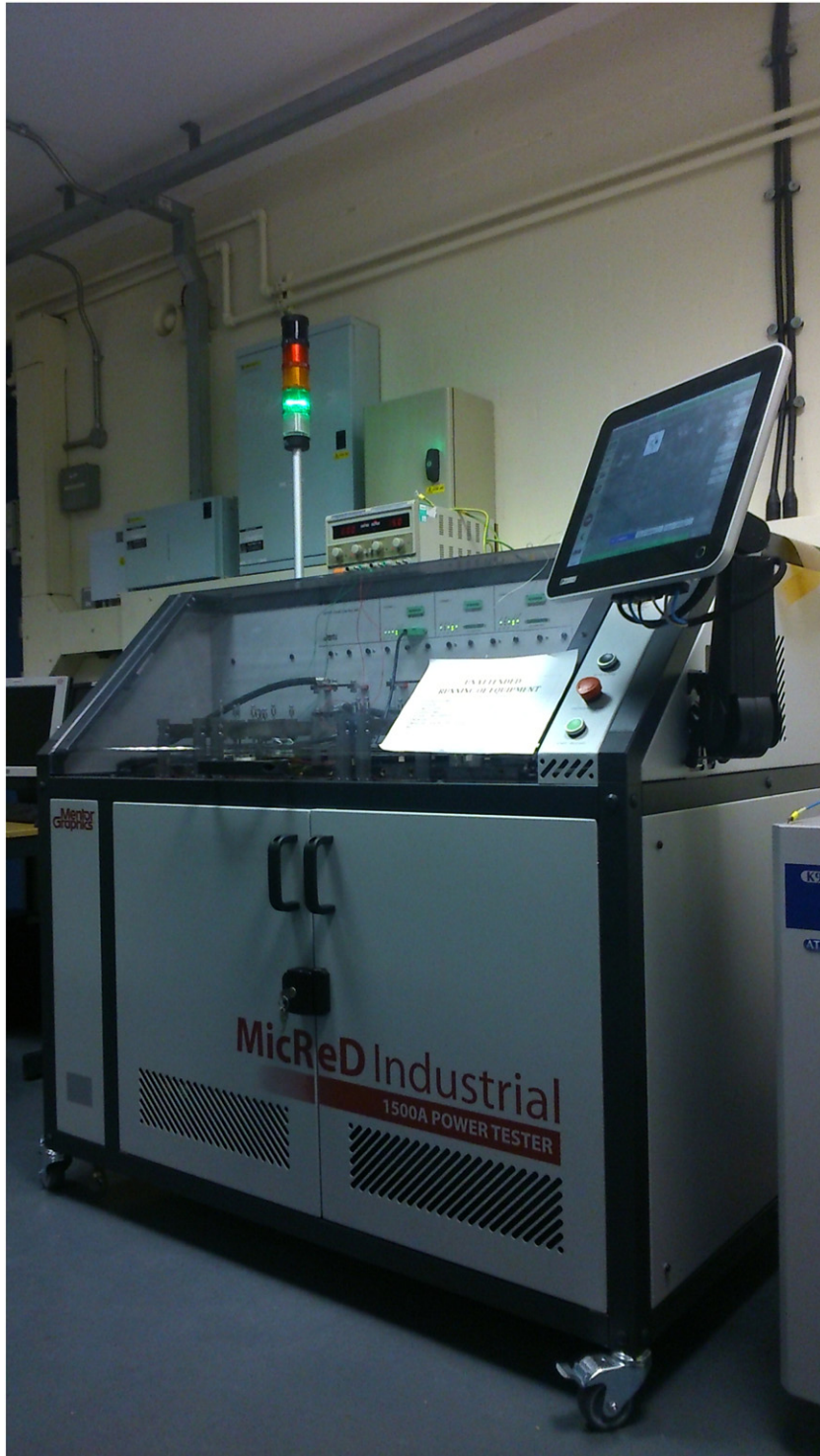
Fig. 1. Mentor Graphics Power Tester 1500A used for power cycling test.
