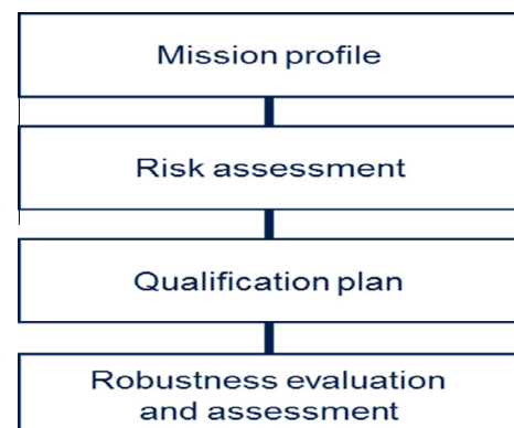
Fig. 3. Reliability assessment flow for Robustness Validation.
