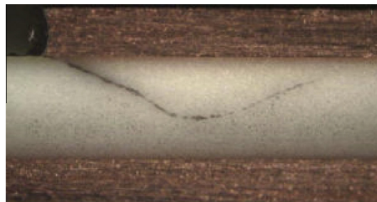
Fig. 1. Conchoidal cracking in DBC ceramic [14]. Crack is initiated at the copper edge and propagates within \text{Al}_2\text{O}_3 .
