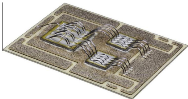
Fig. 1. Typical power module with an IGBT and two diodes connected as a half-bridge circuit [4].
