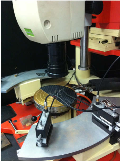
Fig. 1. Probe station equipped with an IR camera for on wafer temperature mapping.
