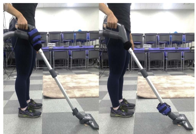
Fig. 2. High CoM model (left) and low CoM model (right), prepared using a canister cleaner wand and a weight sandbag.
