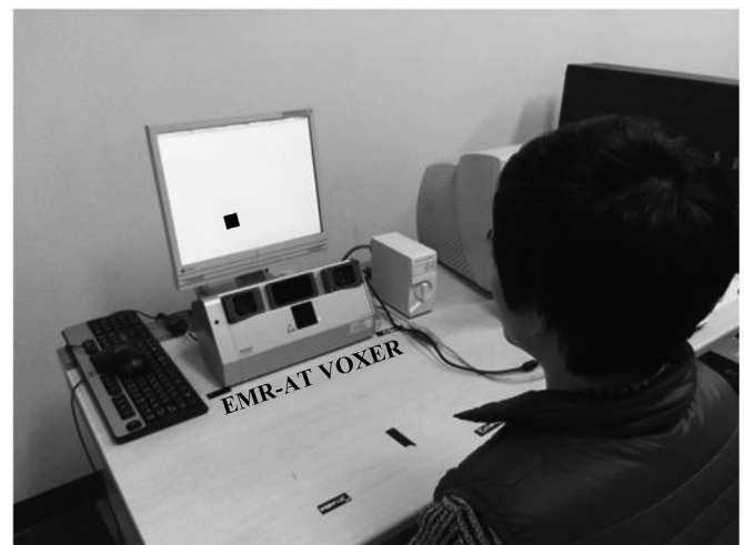
Fig. 1. Outline of experimental setting using an eye tracker (EMR-AT VOXER).
