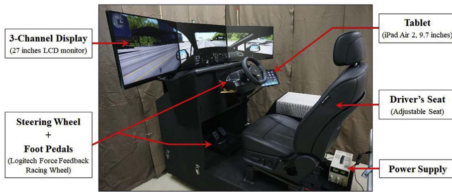
Fig. 1. Setup of the fixed-based driving simulator.
