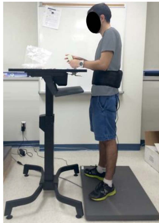
Fig. 1. Image of experimental set-up. Note that in this figure, the belt is over top of the clothes in order to see the location of the belt on the low back. However, for collections, the belt was worn under the clothes against the individual's skin. The vibration motors are only located within the portion of the belt that is up against the low back region and not in the straps of the belt that wrap around to the abdominal region.
