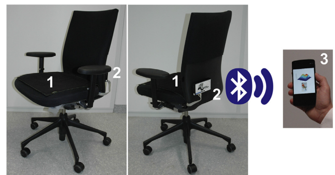
Fig. 1. Schematic drawing of the SIT-CAT sensor system with the textile pressure sensor mat (1), the data acquisition/transmission unit (2) and the mobile phone (3).
