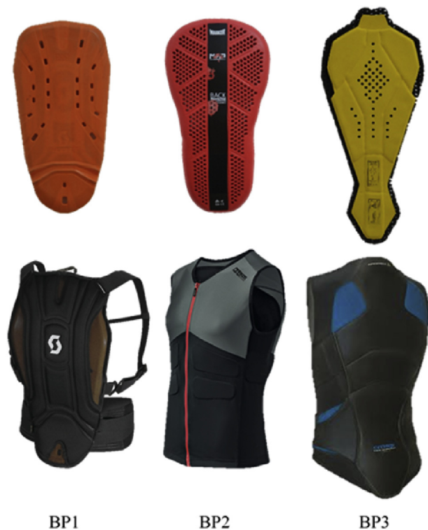
Fig. 1. Soft-shell back protectors tested in this work.
