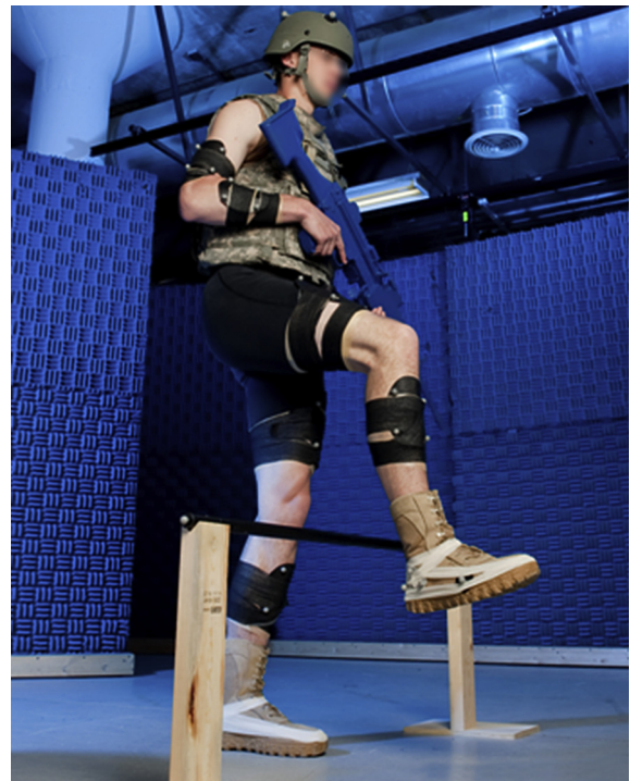
Fig. 1. Equipment for the loaded configuration (~19.4 kg) while crossing the high obstacle (457 mm) is presented. For the unloaded configuration (~6 kg), the participant only wore the helmet and boots, and carried the mock weapon.
