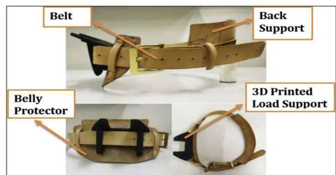
Fig. 1. Prototype of the hip load-carrying belt (HLCB); side view (top); front view (bottom left), top view (bottom right).
