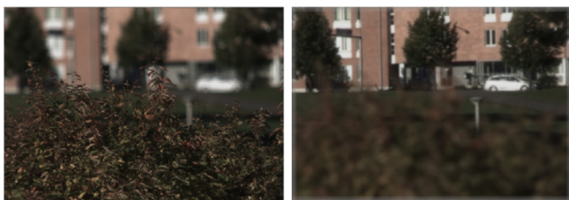
Fig. 1. Digital refocusing of standard plenoptic camera. Left: refocusing with \rho = -1.0 . Right: refocusing with \rho = 1.0 . Without a proper model, the real metric in-focus distance corresponding to each image is unknown.
