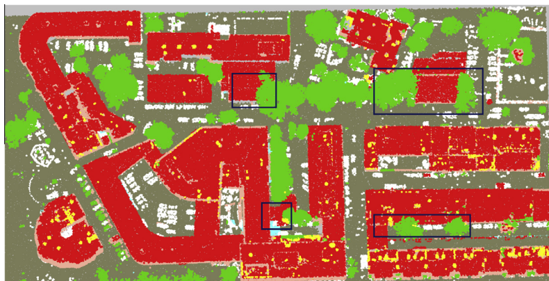
Fig. 1. Example of an urban scene. Many roofs are covered by vegetation in this area, roof elements and vegetation are not easily distinguished, as they both contain multiple pulse returns and have mutable shapes and sizes.
