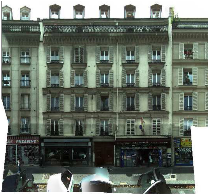
Fig. 1. Typical radiometric issue arising when texturing a building facade (bottom band is darker).
