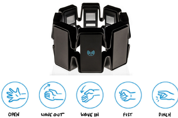
Fig. 2. The Myoarmband integrates 8 EMG channels and an IMU unit and can detect up to 5 gestures.
