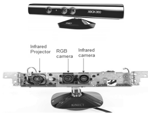
Fig. 1. A Kinect sensor including an RGB camera, an IR projector and an IR camera [10].
