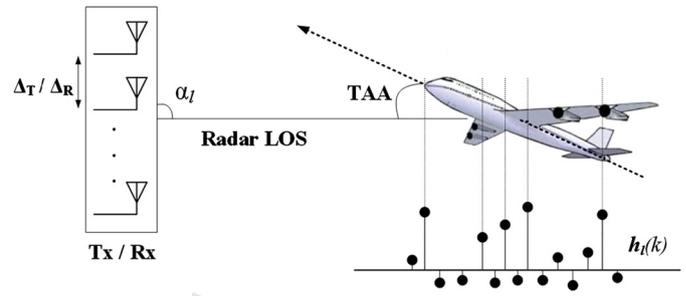
Fig. 1. Returns from the extended target can be represented by several scattering centers projected on the LOS of MIMO radar.
