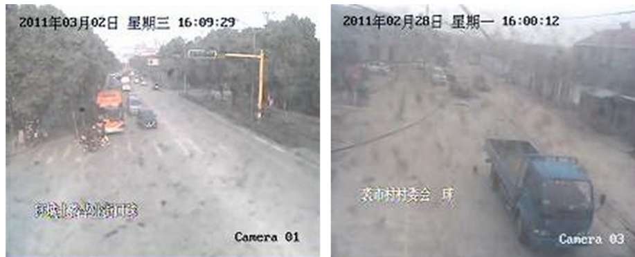
Fig. 1. An example of dust-degraded videos. The objective of dust particle detection in video is to automatically make a decision whether the video is degraded by dust or not.
