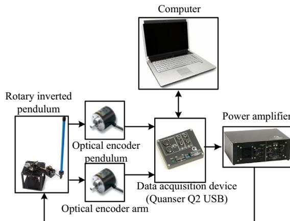
Fig. 1. Schematic diagram of the experimental setup of the RIP.
