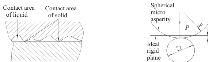
(a) The simplified diagram of the surface contact (b) The contact deformation sketch of the micro asperities
