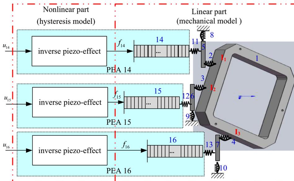
Fig. 2. Schematic comprehensive model of the piezo-stage.
